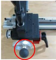
4. Loosen the two black fence lock knobs. Slide the fence on and tighten both knobs.
