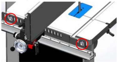
Note: Do not place the fence mounting bracket over blade changing slot in table.
