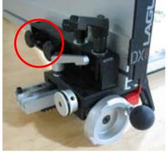
The fence can be repositioned to the horizontal position by loosening the two fence lock knobs.
