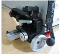
The fence can be moved quickly by releasing (lifting) the lock lever for micro adjustment (A) and extending the red slider (B). To return to micro adjustment mode, check that the red slider is seated and engage the lock lever (C).
