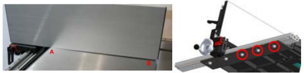
Note: If the rail and infeed side of the fence cannot be raised enough with this adjustment, the mounting brackets attached to the front of the table should be raised.
