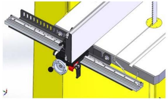
1. Attach both brackets to the table using two bolts. Finger tighten the bolts.
