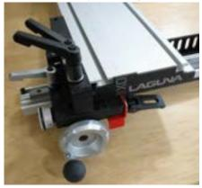
The fence can be moved left and right rotating the handwheel after loosening the fence travel lock. Lock the fence travel lock after choosing the right position. One handwheel rotation moves the fence approximately 7 mm.
