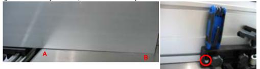
Check to confirm the fence is perpendicular to the top of the table (90°). If not, follow adjustments below.
